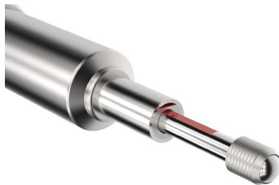
The option VH should be chosen, if the sensor is used in liquids (oil, water, ...) or if fast pressure variations may occur. By milling plane surfaces on parts of the mechanics (see picture red marked) the pressure balance or venting of the inside area will be improved.
