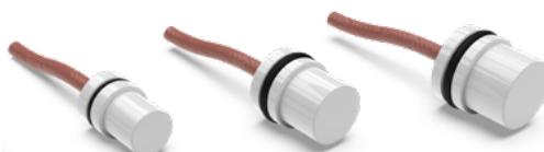
The CM Series are eddy current sensors, excellent for use in harsh industrial environments under high pressure and temperature conditions. The ceramic housing can be used as the pressurised component, there is no extra housing needed. All CM sensors are shielded. The combination of shielded coil and ceramic housing guarantees an universal use in limited space of machine parts. Measuring of lubrication gap of crankshafts is a typical application for the CM series.
