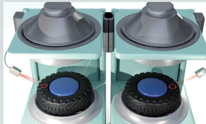
Controlling heating time in tire vulcanization processes
