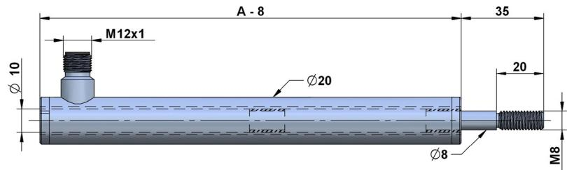
push rod supported by Iglidur bearings, push rod completely extricable
