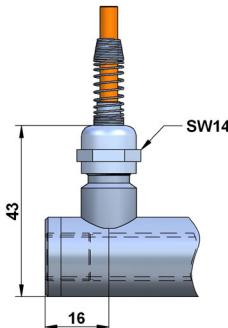
Sensors with cable output have a cable fitting and a spring for bend protection of the cable. For installation, the bending radius should not be less than 3 times the cable diameter. The standard cable length is 2 m.
