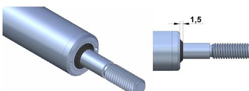
Sensors with guided push rod (type „SG“) or rod end bearings („G“) can be equipped with a wiper ring to prevent the penetration of dust, dirt and metal swarf.
