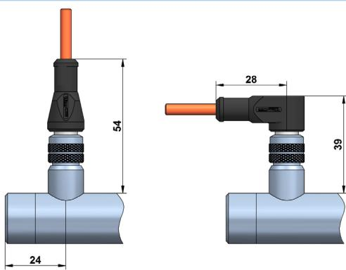
For sensors with connector output the cable has to be ordered separately. You can choose from a cable with a straight connector or with an angular connector.
