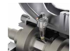
Inspection and part quality analysis during production in the presence of cooling lubricant. Detection of gearing. Groove detection. Detection of flat portions on shafts.
