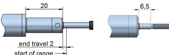
A special design of a fluorocarbon sealing is integrated in the sensor front cap. It combines sealing and wiping and ensures a smooth motion of the mechanics.
