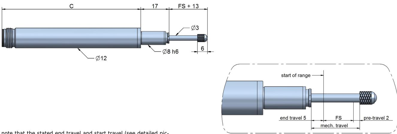
Please note that the stated end travel and start travel (see detailed picture) are standard values. When calibrating the sensors we are aiming for best linearity.
