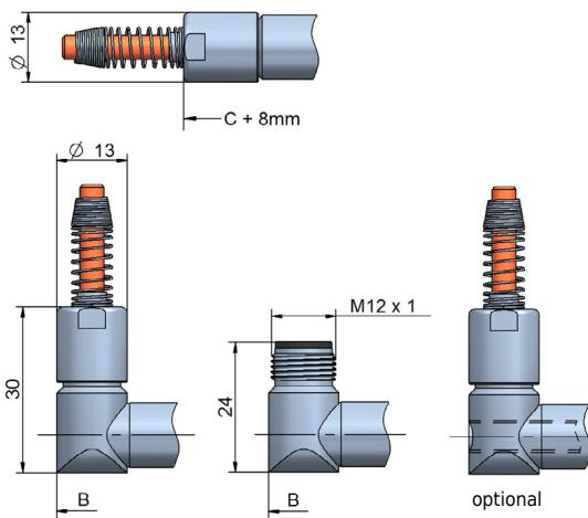
Sensors with cable output have a cable fitting and a spring for bend protection of the cable. For installation, the bending radius should not be less than 3 times the cable diameter. The standard cable length is 2 m.
