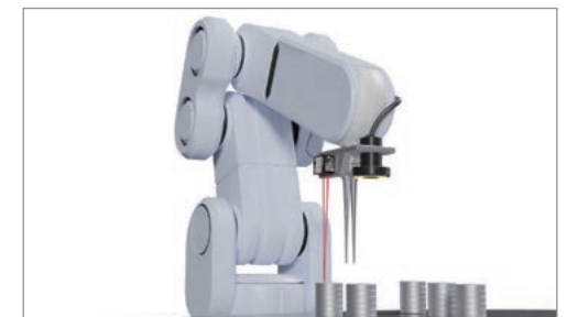
Stacked Bearing Height Measurement
