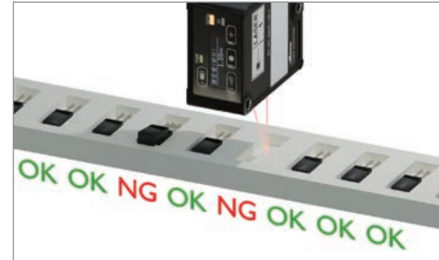
Detecting Seal Material on Pressed Products
