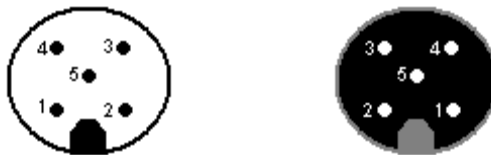
Figure 8: Pin code: Connection plug / socket for 5-pin version
