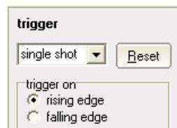
In the mode »Free Run« the measuring values are displayed in an continuous way. In the mode »Triggered« writing starts, when the distance value exceed a trigger level. The presentation ends with reaching the right window margin and starts only then, when the above mentioned condition comes true.
