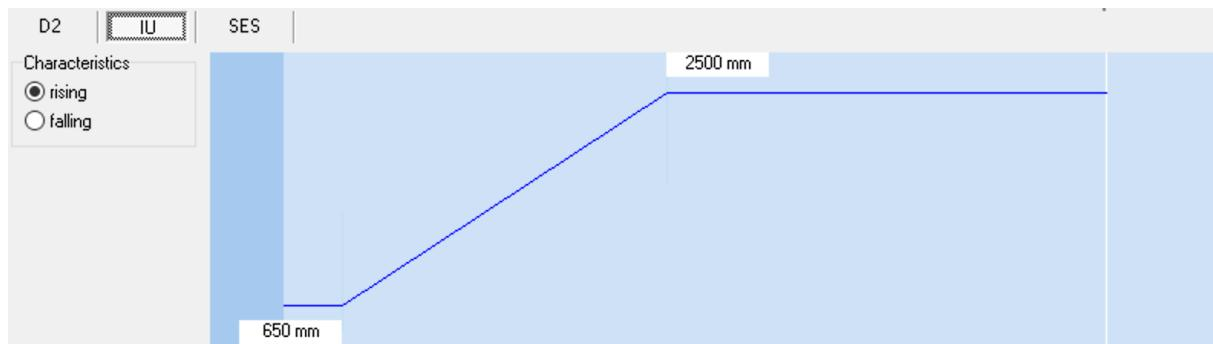
The ultrasonic sensors with analogue output transmit the measurement as a proportional voltage (0-10 V) or current (4-20 mA). For ultrasonic sensors with analogue output, the near and far window boundary of the analogue characteristic and also whether the characteristic is rising or falling can be configured. Depending on the sensor type and window width, resolution lies between 0.025 and 0.36 mm.
