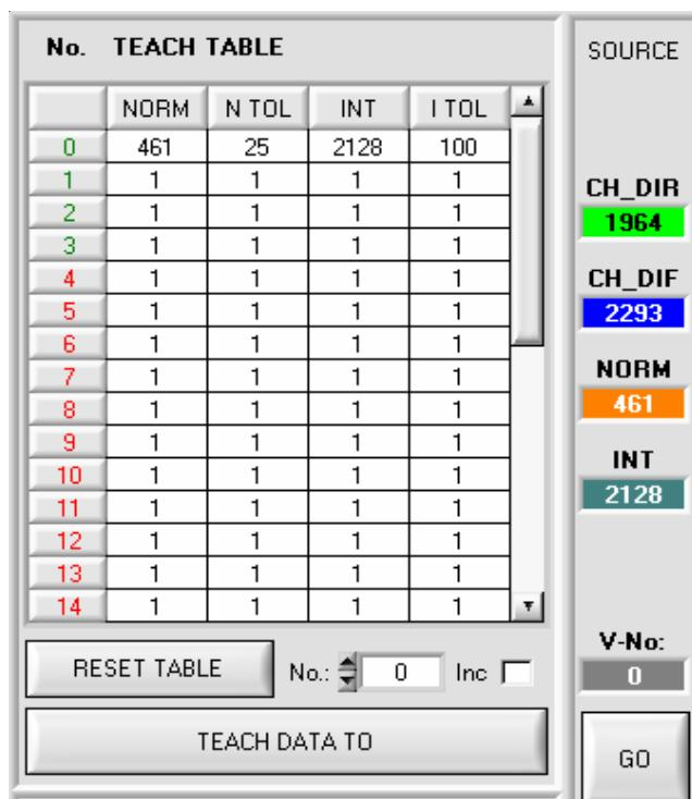
SOURCE is used for selecting which signal (NORM or INT) should be shown in the graphic display. In addition to the signal, the tolerance window that was selected under No.: is also displayed.
