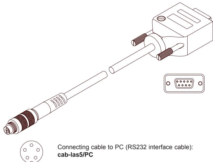
Connecting cable to PC (RS232 interface cable):
