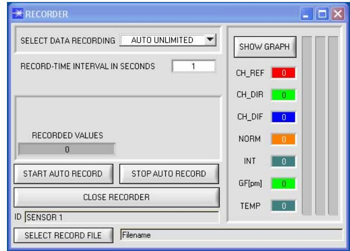
If you want to record data "manually", please select the MANUAL RECORDING function under SELECT DATA RECORDING. You can start reading data from the sensor by pressing the START POLLING button. These data are visualised in the display window. Pressing the CAPTURE DATA FRAME button saves a data frame in the file that was selected under SELECT RECORD FILE. The RECORDED VALUES field shows the sum of the frames already recorded.
