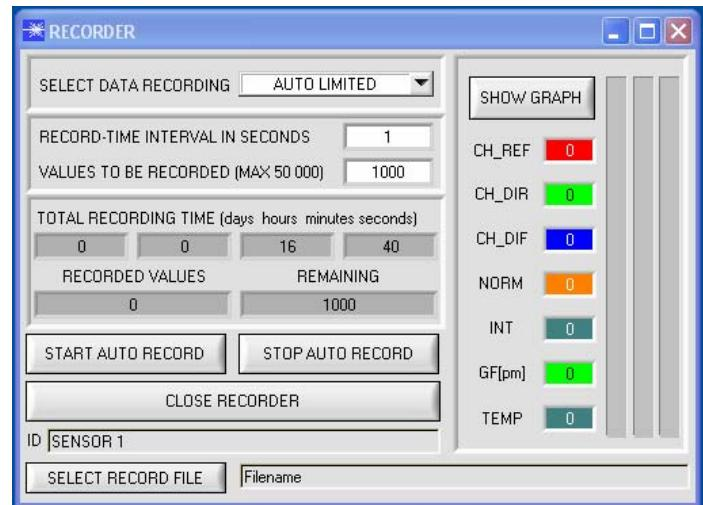
If you want to record an unlimited number of data, please select the AUTO UNLIMITED function under SELECT DATA RECORDING. Select the desired recording interval and press START AUTO RECORD.
