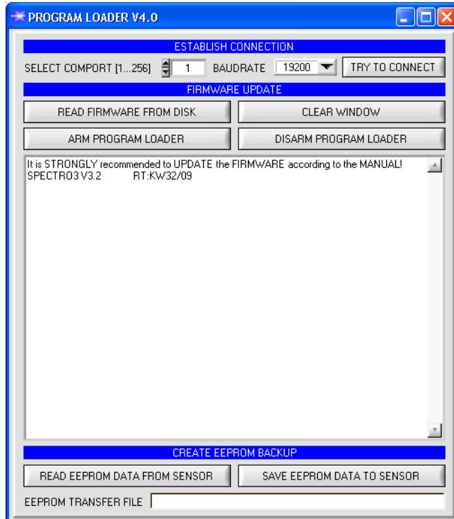
The software „Program Loader“ or „Firmware Loader“ allows the user to perform an automatic firmware update. The update will be carried out through the RS232 interface.
