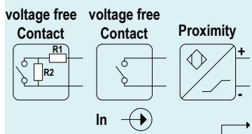
Resistors R1 - R2 used with voltage free contact required for line fault detection.
